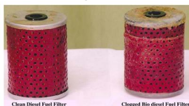
Fig.2. Filter clogging with 100% MME
